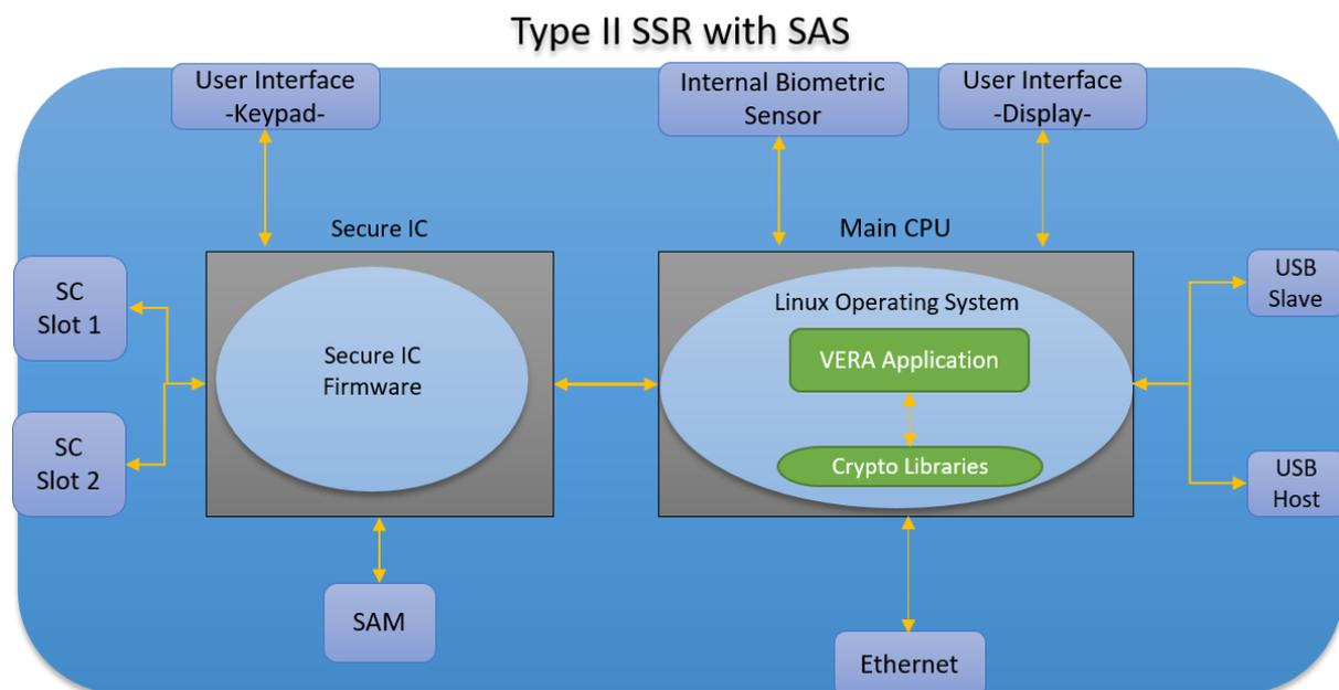
**Figure 4. Physical Scope of the TOE Software**
